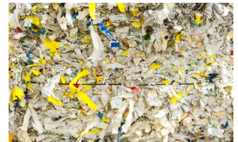
KP utilizes sorted office waste as its primary input in creating recycled fibre. The waste is de-inked and pulped in our Crabtree, QC plant.
